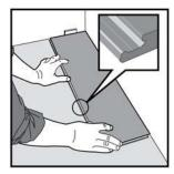
**1.** First plank, first row. Place a distance  $\frac{1}{2}$ " (5mm) thickness to the left and position the plank against the wall. Later, after 3 rows, you can easily position the flooring against the front wall with distances  $\frac{1}{2}$ ".
