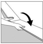
**2.** Second plank, first row. Press the short end of the next floorboard at an angle to the first one, and then lay down. Complete the first row in the same way.
