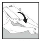
**7.** Second plank second row. Place the short end of the floorboard at an angle against the previous installed floorboard and fold down all the way.
