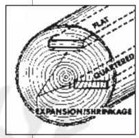
The ideal moisture content for flooring installation can vary from an extreme of 4 to 18 percent, depending on the wood species, the geographic location of the end product and the time of year. Most oak flooring, for example, is milled at 6 to 9 percent. Before installation, solid wood flooring should be acclimated to the area in which it is to be used.
