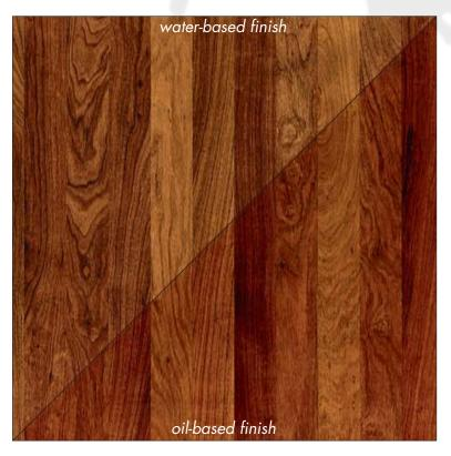
**COLOR:** Light brown to dark reddish brown. **GRAIN:** High in character, with ingrown bark and mineral streaks. Most commonly used in flooring as end-grain block, which has small irregular cracks radiating across the grain. **VARIATIONS WITHIN SPECIES AND GRADES:** One
